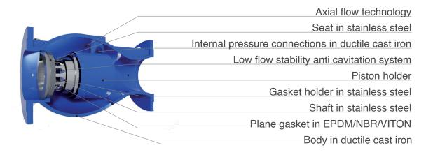
The mobile block includes the obturator, shaft and gasket holder, the latter engineered with different versions to guarantee the maximum accuracy and best performances in accordance to the results of the sizing, resistance to cavitation and design requirements.
