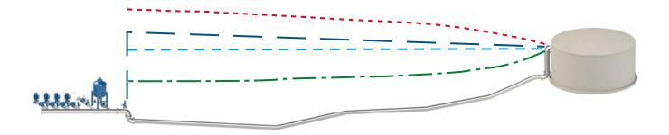
The plot above shows the pressure envelope of the transient event caused by pump failure on a pipeline with SPT. installed as a protection. The red and green are the maximum and minimum pressure values reached during the simulation, it is clearly visible the beneficial effect in terms of negative pressure and consequently reduction of water hammer.
