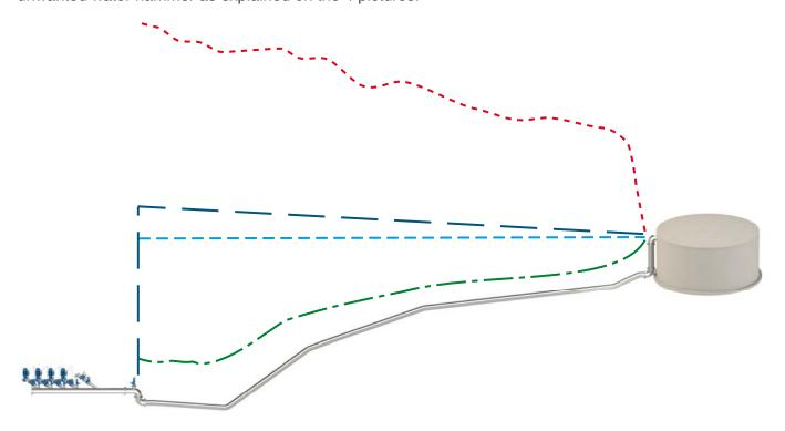
The results of pump failure can be summarized in a plot showing the envelope of the maximum and minimum pressure values reached during the simulation, in the picture above shown respectively in green and red. It is evident how the system reaches a full vacuum on the entire profile and an extreme rise in pressure due to the column separation, occurred at the change in slope.
