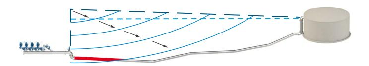
The plot above shows a pipeline profile, with pumps and downstream tank as boundary conditions, where the dark blue dotted line represents the HGL and the light blue dotted line is the static. The picture represents the negative pressure wave propagating downstream as an effect of pump failure, where the red segment depicts the area exposed to negative during the initial phase of the event.
