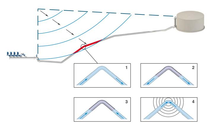
The plot above shows the negative pressure wave propagating downstream, as an effect of pump failure. The red segment depicts the area exposed to severe negative pressure. The change in slope represents a location at risk of column separation, caused by vapour pockets forming and then collapsing creating unwanted water hammer as explained on the 4 pictures.
